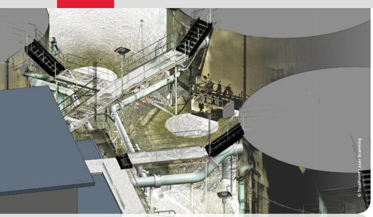
A colourised point cloud of the water treatment plant with modelled tanks and building footprint.
