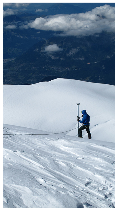
Using a Leica Viva GS14 antenna to measure and calculate the volume of the ice cap to create a 3D model.
