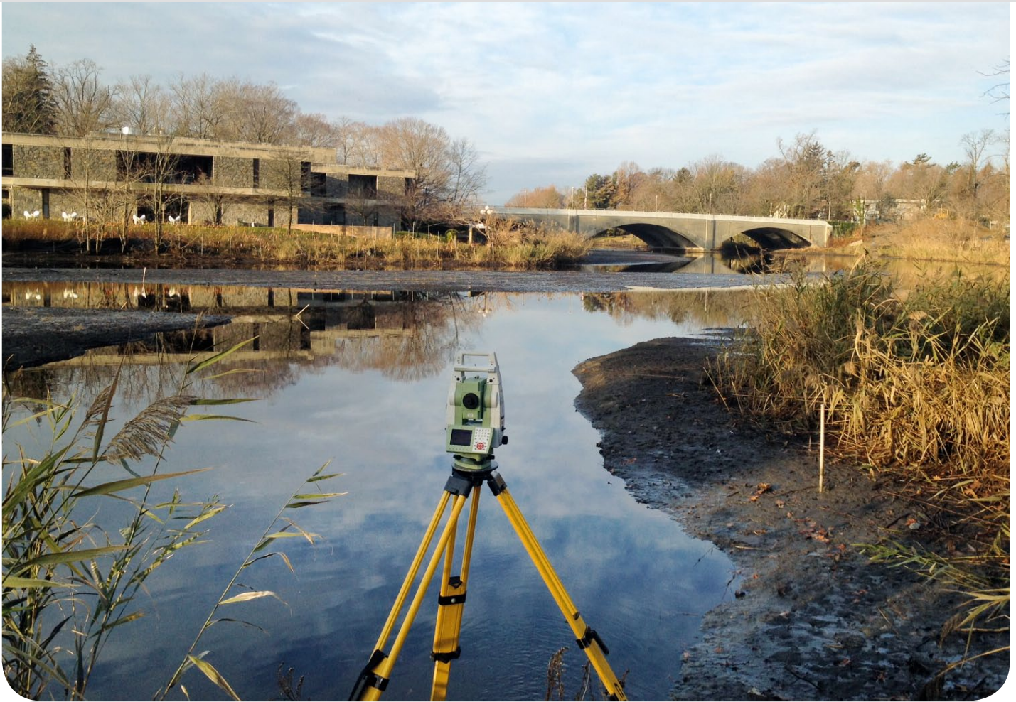
■ A Leica Viva TS15 is used to survey Udalls Pond in Nassau County to determine the sedimentation effects of Sandy.
