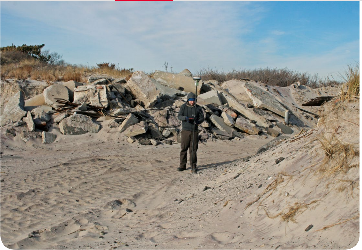
■ A GdB field crew uses a Leica Viva GS15 to survey post-Sandy beach erosion for the town of Oyster Bay.
