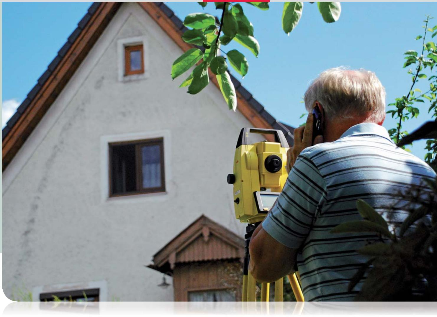
the possibilities offered by the Leica Builder. By the time he left the site, he had made himself familiar with the instrument's simple and logical operation. With reflectorless distance measurement and user-friendly programs at his disposal, all Staudt has to do is capture the corner points of the roof from the eaves to the ridge to immediately obtain the area and even the inclination of the roof.
