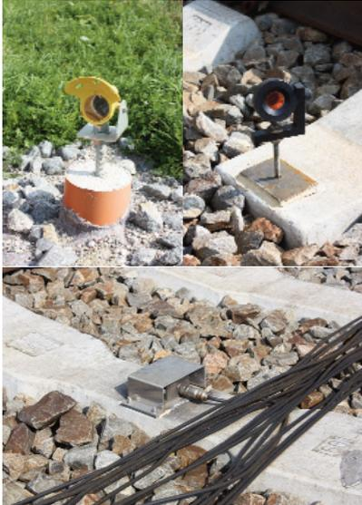
Leica GPR112, Leica GMP104 prisms and tilt sensor
