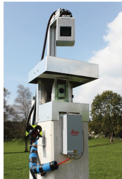
Measurement pillar with Leica TM30 and webcam
