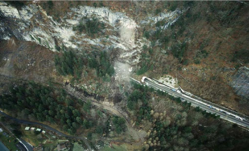
**In January 2003 there was a fall of approximately 150 m<sup>3</sup> of rock from above the Chüebalm tunnel in Iseltwald/Interlaken. The falling rock punctured the tunnel near the western entrance and blocked the highway.**
