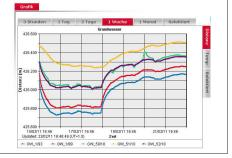
Graph of the groundwater level in Leica GeoMoS Web
