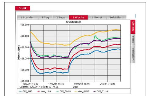
Graph of the groundwater level in Leica GeoMoS Web
