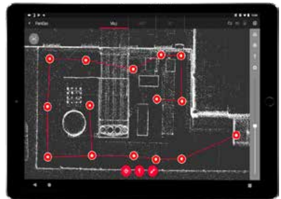
Auto-aligned point clouds in 2D view mode
