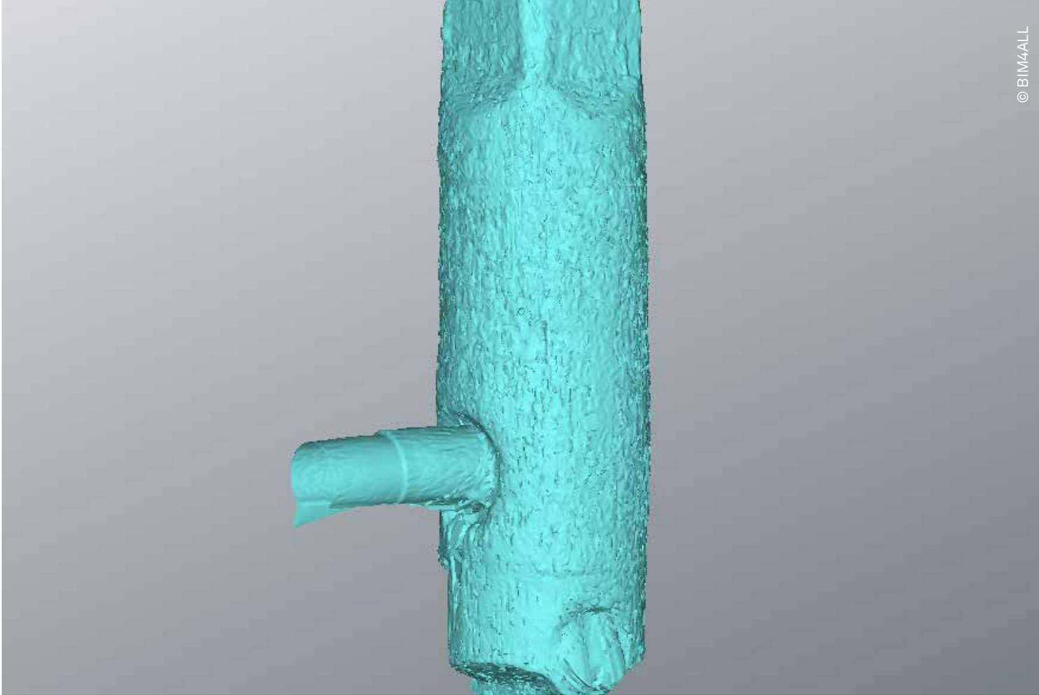
The detailed scans were processed in Leica Cyclone point cloud processing software then exported using the Leica CloudWorx for 3D Reshaper plugin to visualise meshes for the client's review. This reduces noise in the point clouds, enabling clients to clearly see the corrosion in the pits and allowing them to precisely create the needed composite moulds.
