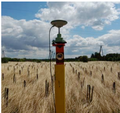
New Reference Station outside of the movement area.
