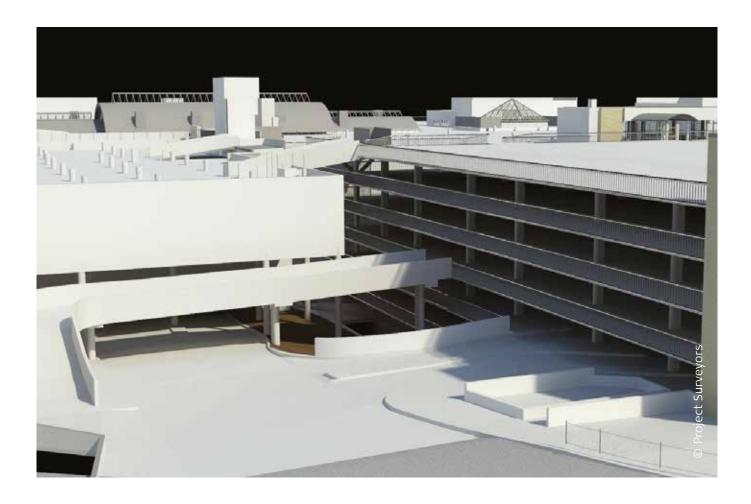
The Sydney shopping centre is currently undergoing redevelopment, and the client needed a fully-parametric Building Information Modelling (BIM) model for architects, engineers and facility managers to accurately plan the work needed. Covering a space of 375,000 square metres with various dimensional obstacles, such as cascading floors, topographic level changes and add-on buildings of diverse sizes, Project Surveyors faced one of its most complex jobs in its 43-year history.
