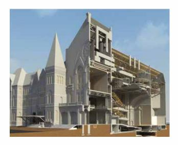
preconstruction as-builting, construction layout, and quality assurance as-builting. It's worth noting that the MultiStation introduces a new era of versatility in BIM workflows with the ability to use a single instrument for pre-construction as-built point cloud data capture, replicating highly accurate BIM layout points in the field, and then high-definition laser scanning for quality assurance as-builts for comparing with as-designed models to create a complete 3D BIM lifecycle.
