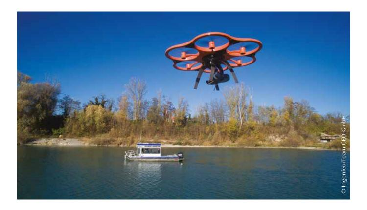
Focusing on surveying engineering technologies, IngenieurTeam GEO was contracted to determine the remaining volume in Knobel-Bau's quarries. By creating georeferenced orthophotos and digital terrain models using the Aibotix Aibot X6 unmanned aerial vehicle (UAV), the firm was able to present the current situation in detail and provide an effective inventory reduction plan.
