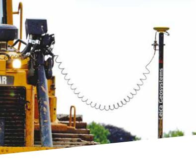
Leica Geosystems Machine Control GNSS solutions have played a major part in the Walters armoury with the aforementioned excavator and four new D6T dozers resident on the site fitted with the Leica iCON iGD4 3D system. Working with GNSS reduces the need to have engineers out on site working in close proximity with moving vehicles and does away with the large amount of timber pegs and rails that have to be installed.
