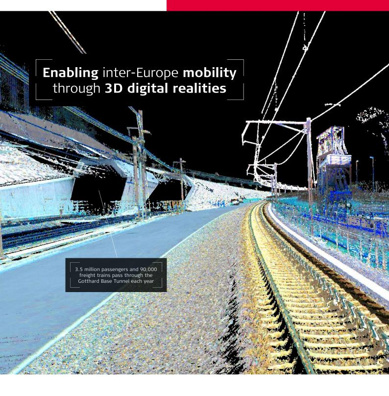
Leica Pegasus:Two mobile mapping technology enabled Grunder Ingenieure AG to efficiently capture the as-built environment of the Gotthard Base Tunnel in Switzerland in only a few weeks, without disrupting the ongoing construction, benefiting all working stakeholders.
