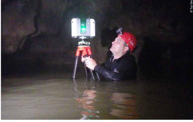
DISTO™ data, too. Together with Spelemat, Top Geocart created a unified point cloud, as Cyclone REGISTER 360 project, and exported in E57 and LGS formats to visualise it with JetStream Viewer, a light-weight point cloud viewing tool. The E57 file was imported in Leica Cyclone 3DR to create meshes and compute digital terrain models (DTM) from point clouds.
