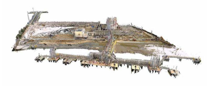
data. After collecting the point cloud data from the geodetic equipment, Portcoast used Leica Cyclone, Leica Cyclone 3DR and Leica Infinity software off-site to process the data.
