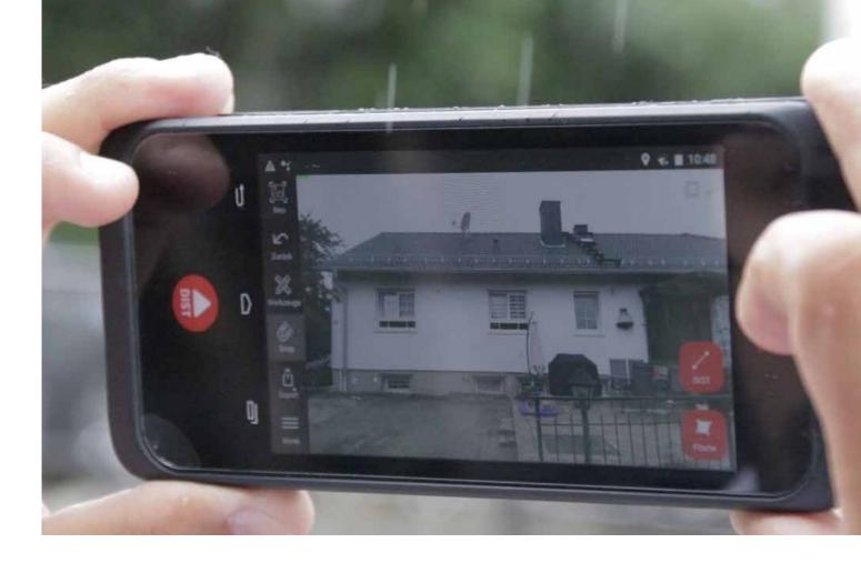
check, but variations between this and the in-picture measurements are usually less than 1 centimetre. If the process is followed correctly, meaning two images are taken, which are then overlaid, the accuracies are more than satisfactory for a scaffolder. For the final invoice, however, measurements of the actual installations are used.
