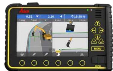
Run screen for excavator with swing boom
