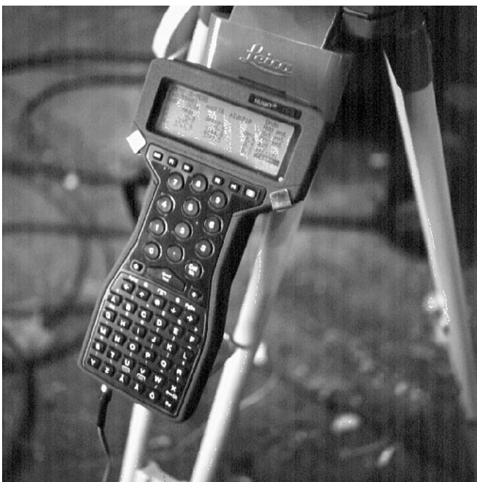
Picture 2: The field computer with the on-board DCP10-software
