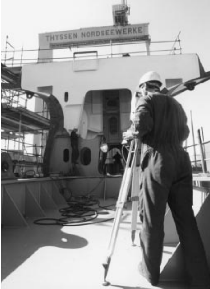
Picture 1: The DCA-TPS system in action at Thyssen Nordseewerke
