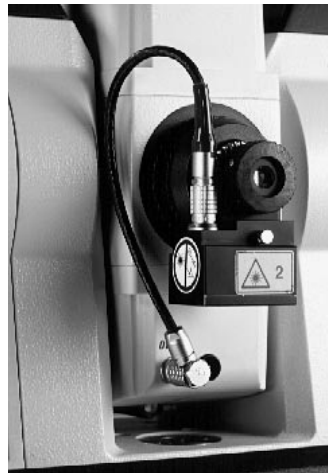
Picture 8: Laserpointer DL2 to visualize the 3D location on site according to design data
