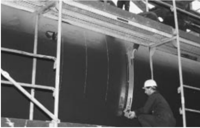
Picture 5: Conventional, staff intensive method for roundness checks using a gauge (1D measurement)
