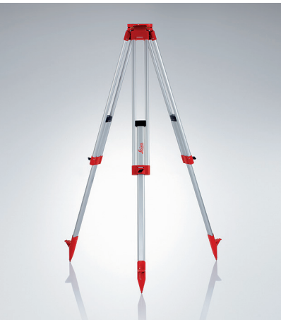
GST05L, Aluminium tripod Light duty tripod with shoulder strap. Light-weight and long lasting making it suitable for GNSS antennas, prisms and levels. Packaged length 107 cm (3.51 ft), extendible to 176 cm (5.77 ft), weight 4.6 kg (10.1 lb). Order No: 563630
