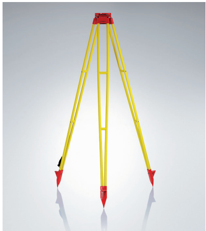
GST40, Wooden tripod Heavy duty tripod with rigid legs, suitable for precision levelling. Proven long-life, twist-proof and excellent vibration characteristics. Length 170 cm (5.58 ft), weight 6.0 kg (13.2 lb). Order No: 328422
