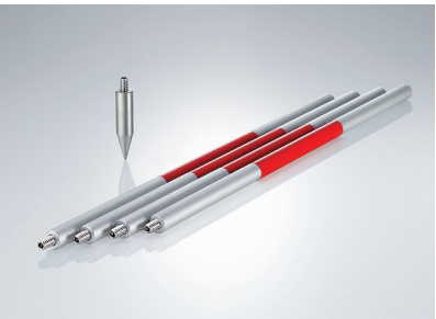
GLS115, Mini pole Set of four screw-together sections and point with 1/4" threads. Suitable for GMP111, GRZ101 and GPR105 reflectors. Provides prism heights of 10, 40, 70, 100 or 130 cm. For prisms without bubble a additional clip on bubble is available (GLI115, 747895). Order No: 642106
