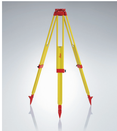
GST20-9, Wooden tripod Heavy duty tripod with carrying strap and side clamp screws. Proven long-life, twist-proof and excellent vibration characteristics. Packaged length 110 cm (3.61 ft), extendible to 180 cm (5.91 ft), weight 6.4 kg (14.1 lb). Order No: 394752
