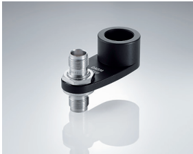
GAD34, Arm 3 cm for UHF/GSM antenna Arm 3 cm long, screws on telescopic rod with 5/8" screw. UHF/GSM antenna fits on arm. Antenna cable connects to arm. Order No: 667220
