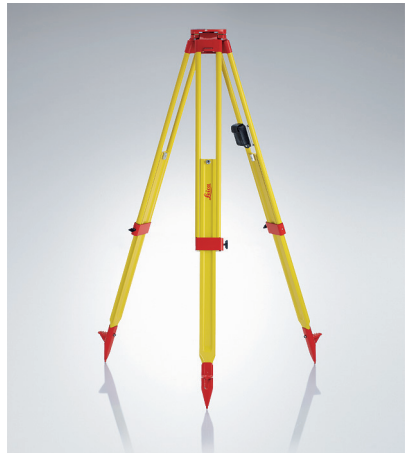
GST20, Wooden tripod Heavy duty tripod with plumb bob, carrying strap and side clamp screws. Proven long-life, twist-proof and excellent vibration characteristics. Packaged length 110 cm (3.61 ft), extendible to 180 cm (5.91 ft), weight 6.4 kg (14.1 lb). Order No: 296632
