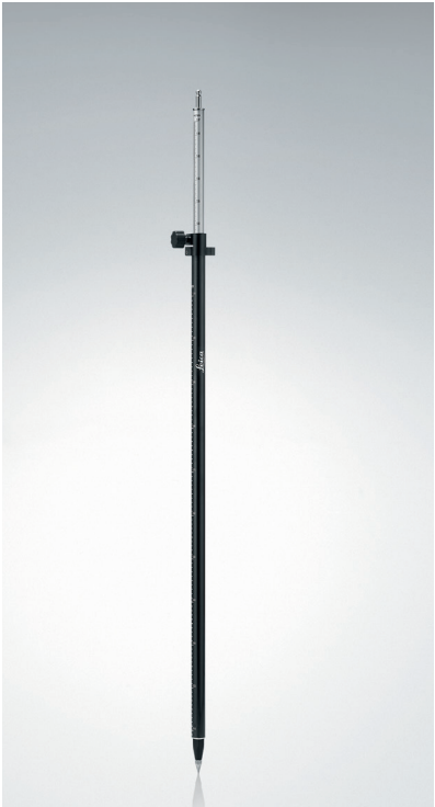
GLS101, Telescopic pole Carbon / aluminium reflector pole with twist lock and pin lock to prevent any pole slip. Graduated in cm and ft. min length 1.31m, extendible to 2.3m, weight 1.230 g. Order No: 865472
