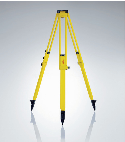
GST101, Wooden tripod Heavy duty tripod with carrying straps and side clamp screws. A cost effective alternative for TPS instruments with angular measurement accuracy starting from 5" and reflectors. Packaged length 104 cm (3.41 ft), extendible to 166 cm (5.45 ft), weight 5.7 kg (12.6 lb). Order No: 726831
