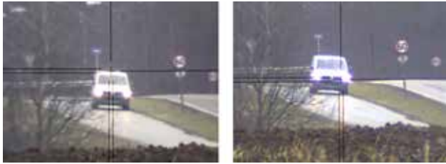
Figure 4 – ATRplus (left) is correctly locked onto the prism on the top of the car. ATR (right) tries to lock onto the car headlights.
