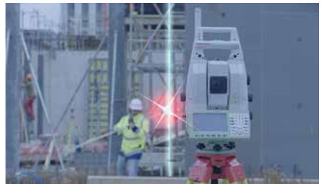
Figure 6 – CubeSearch using Dynamic Lock onto a moving target.
