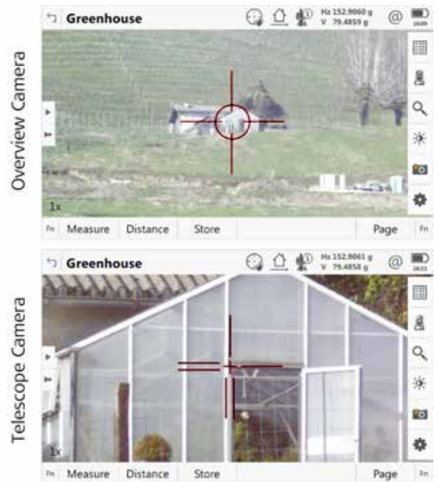
Figure 7 – Scenery displayed with live video stream: once with the overview camera and once with the telescope camera.
