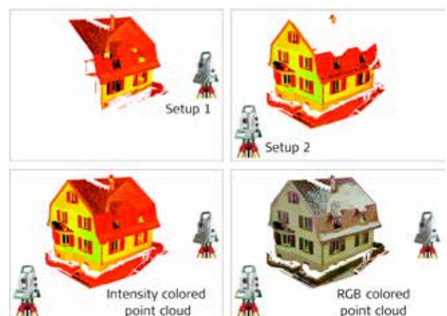
Figure 13 – Auto-registration of the point clouds directly in the field.
