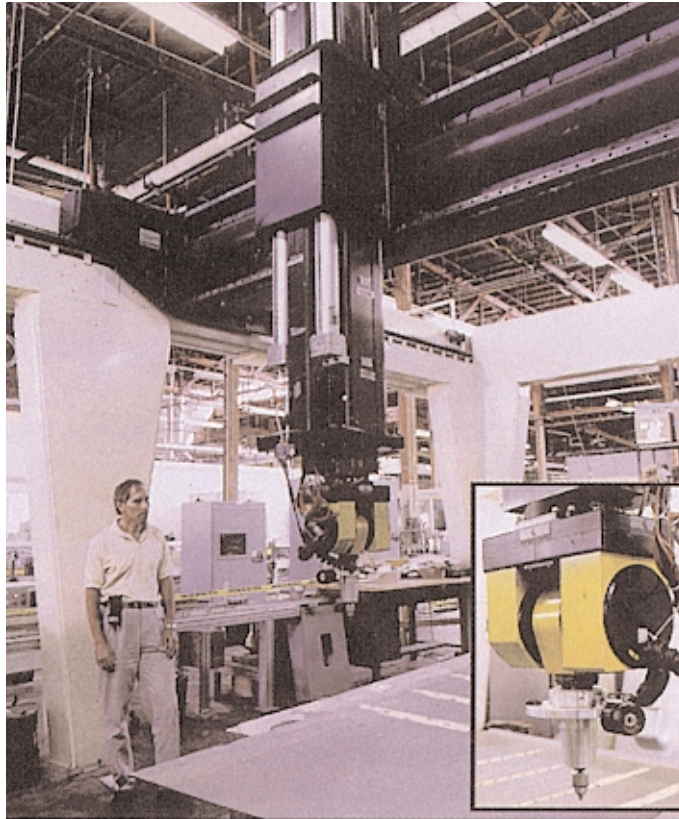
Martin Berg observes the gantry robot test bed in action. Inset: Wrist with retroreflector for the laser tracker
