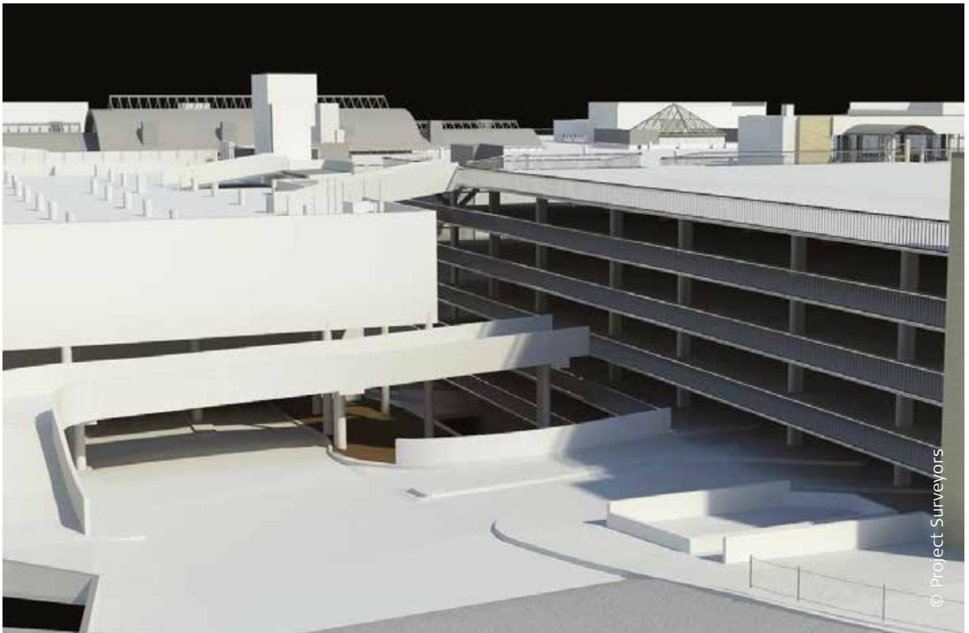
The Sydney shopping centre is currently undergoing redevelopment, and the client needed a fully-parametric Building Information Modelling (BIM) model for architects, engineers and facility managers to accurately plan the work needed. Covering a space of 375,000 square metres with various dimensional obstacles, such as cascading floors, topographic level changes and add-on buildings of diverse sizes, Project Surveyors faced one of its most complex jobs in its 43-year history.
