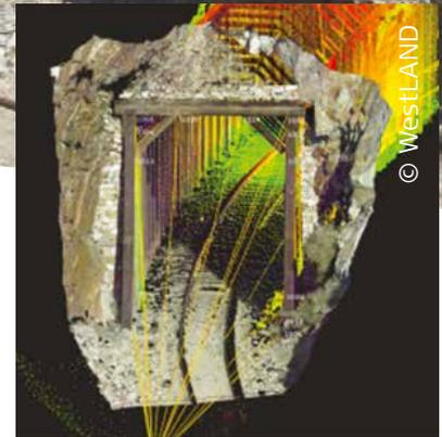
Railroad for use with double stacked trains, and 17 tunnels will have to be surveyed for clearance analysis and possible grading and track redesign. WestLAND saw the scan of one tunnel as basically a marketing investment and offered to scan one of the smaller tunnels, No. 15, which was only 91.4 metres long. It was the first project to make use of the MultiStation and it went very well.
