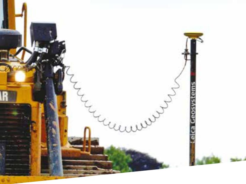
Leica Geosystems Machine Control GNSS solutions have played a major part in the Walters armoury with the aforementioned excavator and four new D6T dozers resident on the site fitted with the Leica iCON iGD4 3D system. Working with GNSS reduces the need to have engineers out on site working in close proximity with moving vehicles and does away with the large amount of timber pegs and rails that have to be installed.
