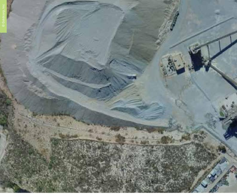
Located in the northeast corner of Zacatecas State, Mexico, Peñasquito is Mexico's largest gold producer, consisting of two open pits -Peñasco and Chile Colorado - containing gold, silver, lead and zinc. Mining (pre-stripping) began in 2010 and full production in 2011. The open pit mines feed both a sulphide concentrator (mill) and a heap leach pad. Peñasquito's project is owned by Goldcorp, Inc. and is a poly metallic deposit with gold, silver, zinc and lead being recovered as payable metals.
