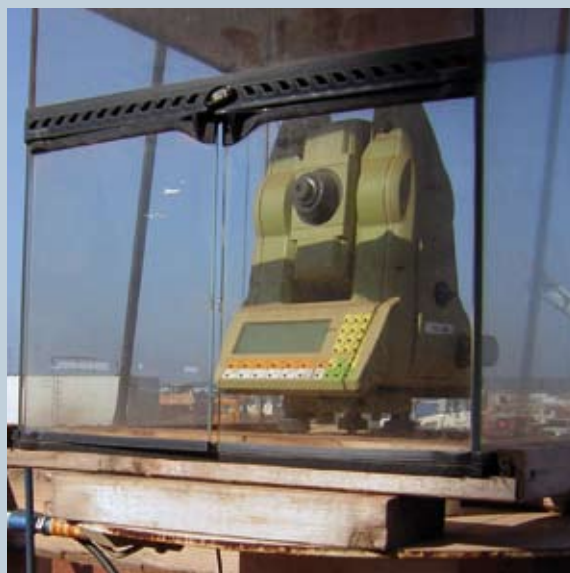
■ A Leica TCA1800 in use at Washington Dulles airport. Picture: Marc Cheves
