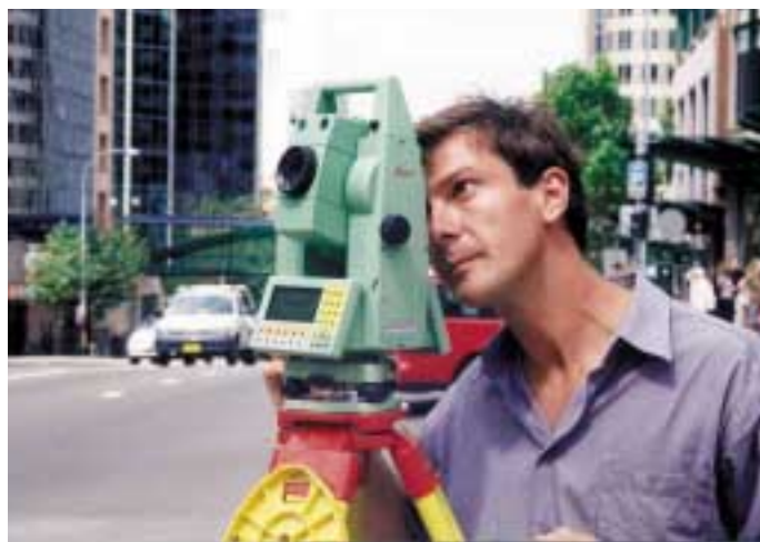
The data collection phase encompassed control measurement using electronic theodolites, first- and second-order GPS positioning and adjustments. Several hundred second-order control stations were placed through the area and tied into the State control network. Over a million points were measured to structure the model.
