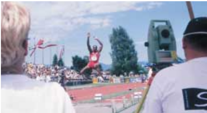
Below: The high jump and discus had already been measured using Leica total stations in the previous year at Götzis using reflectorless techniques.
