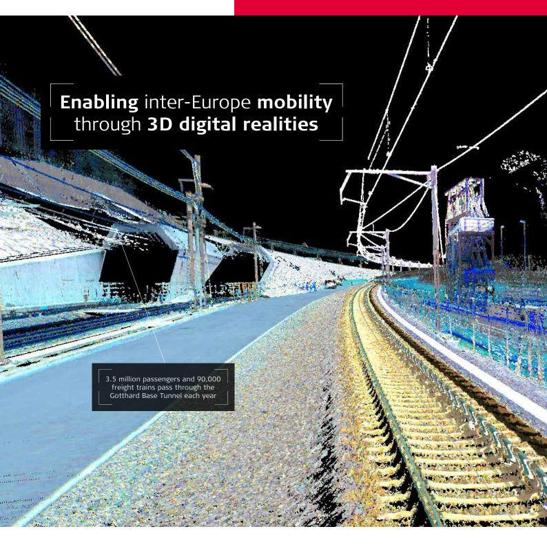
Leica Pegasus:Two mobile mapping technology enabled Grunder Ingenieure AG to efficiently capture the as-built environment of the Gotthard Base Tunnel in only a few weeks, without disrupting the ongoing construction, benefiting all working stakeholders.
