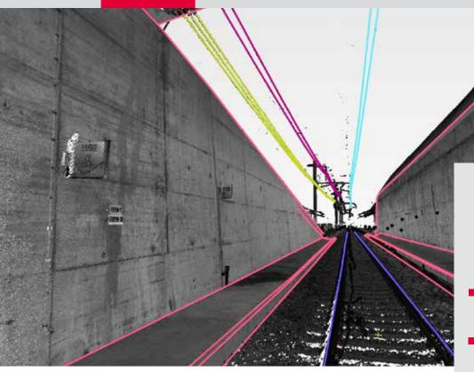
Grunder Ingenieure AG was contracted to deliver a complete inventory and as built documentation of the Gotthard Base Tunnel. Using Leica Pegasus:Two they were able to efficiently capture the entire project in only a few weeks, without disrupting the ongoing construction, benefiting all working stakeholders.
