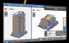
■ Zlider Bar allows you to vertically cut out building model elements for best map visualisation
