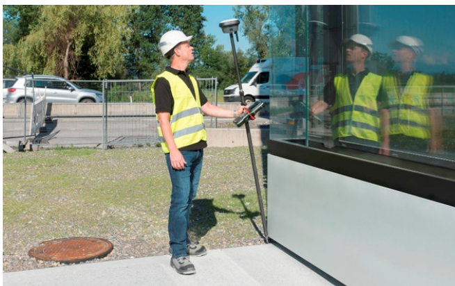
Figure 3 - Using the Leica GS18 T to measure building corners and obstructed points that were previously not measurable in conventional RTK surveying with a vertical pole.
